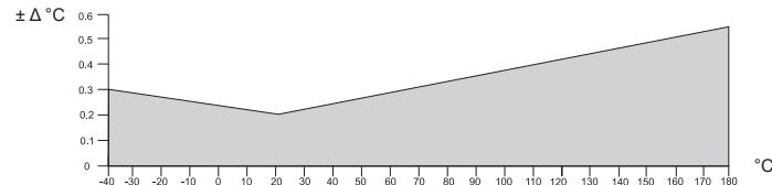
Temperature dependence of electronics, typ. ± 0.005°C / °C
