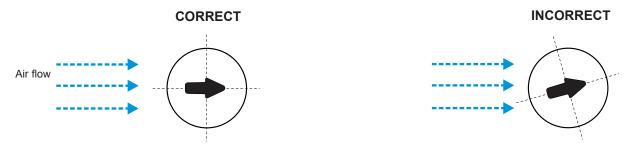
The mounting flange allows for precise setting of the EE650 immersion depth in a duct. The entire sensing head must be in the air flow to be measured.
