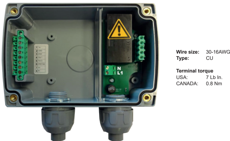
Fig. 13 Option AM5 with liquid-tight conduit fittings
