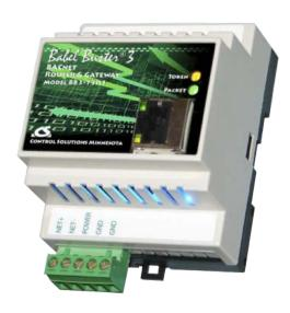
The IAQEye™ is designed to be easily integrated into an existing BACnet control system using a WiFI gateway called the Babbel Buster® that translates the UDP measurement data relayed via WiFi from the transmitter into BACnet® objects used by a control system. Up to 200 IAQEye™ units can be used with one Babbel Buster® (BB3-7302).
