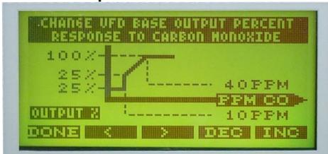
This screen allows adjustment of the VFD response to set different VFD fan speed targets for 4 different target gas concentrations. Here the backlighting is on.
