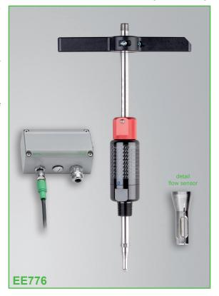
choose between two measuring ranges 0.2...100 Nm/s (40...19685 SFPM) or 0.2...200 Nm/s (40...39370 SFPM) and three different probe lengths with a maximum immersion depth of 165 mm (6.5") / 315 mm (12.4") / 465 mm (18.3"). The inner diameter of the distribution pipe which is measured can be entered via the USB port and the included configuration software.
