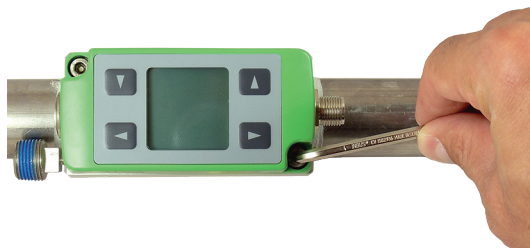
Fig. 11 Tighten mounting screws
